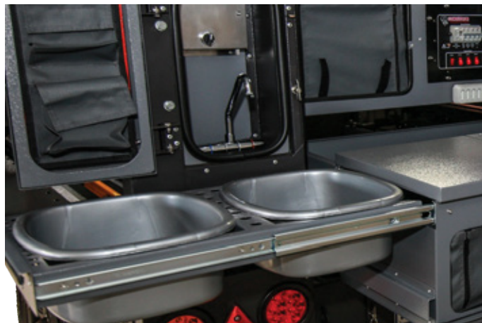
Slide out Dual Basin Tray with instant hot water wash-up facility.
